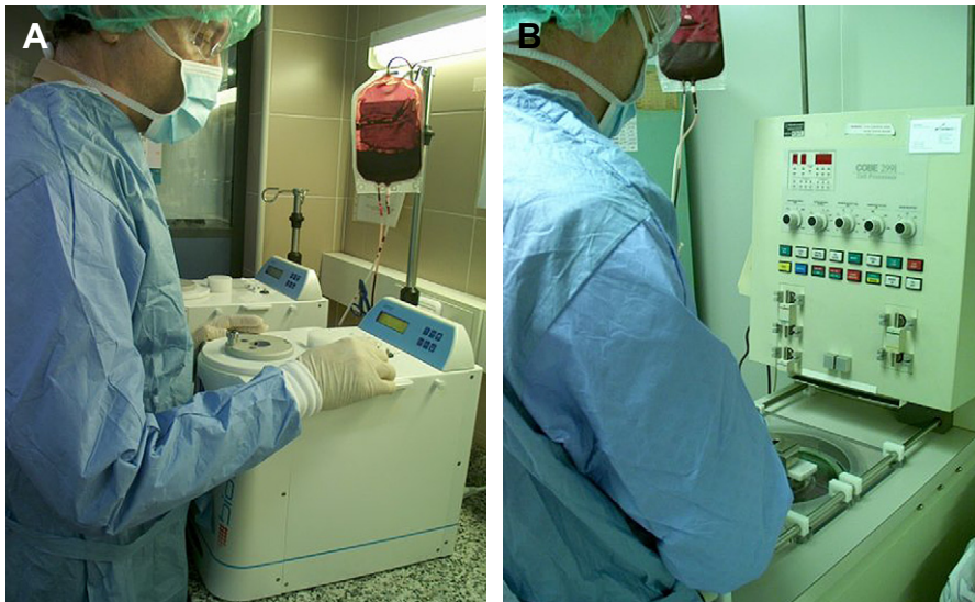
FIGURE 26.5 The use of (A) semi-automated (Sepax) or (B) fully automated (Cobe) devices for centrifugal elutriation reduces cell manipulation. The risk of contamination is thus minimized, which is very important in the case of cells intended for clinical use.
