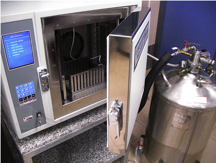
FIGURE 26.8 Controlled rate freezer devices include a freezing chamber, a module with the software for the design and storage of cooling programs, and a container for nitrogen supply, in addition to exhaustive control, data recording and high reproducibility of processing.
