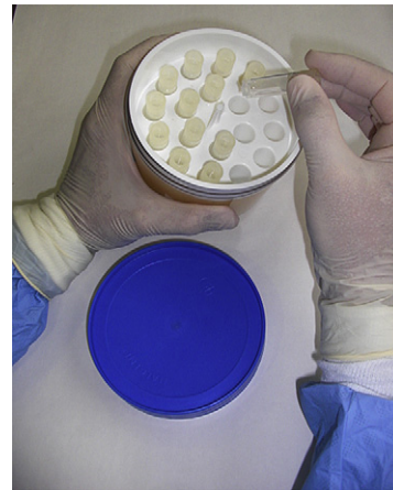
FIGURE 26.9 Passive cooling devices can be used as an alternative for freezing samples near the storage temperature.
