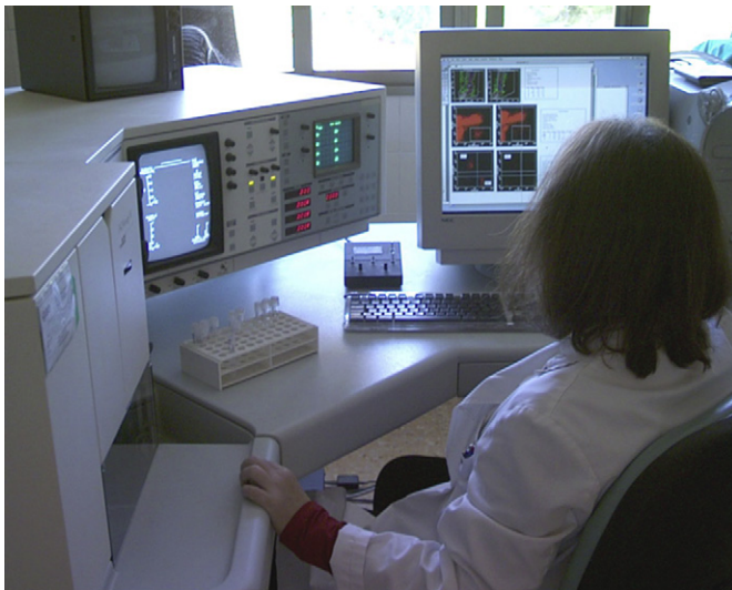
FIGURE 26.7 Fluorescence activated cell sorting (FACS) is a technology developed for counting and examining cell populations. Each cell is individually assessed according to physical characteristics (e.g. size, cytoplasmic complexity) or immunological phenotype (expression of specific antigens on the cell membrane).
